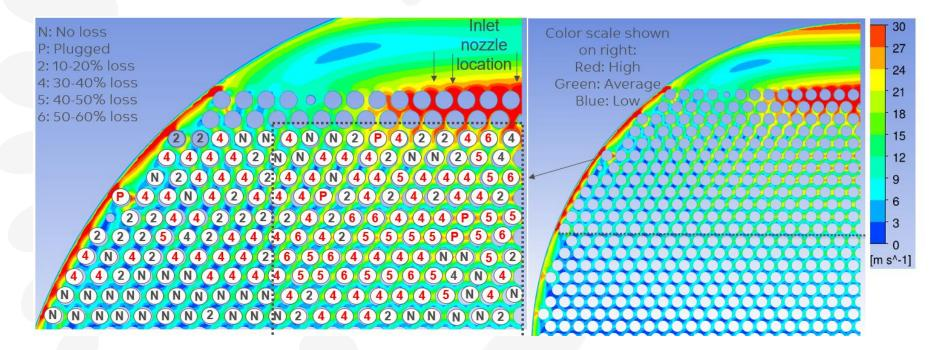
Computational Fluid Dynamics (CFD) Analysis performed to check the flow morphology and determine the flow velocity at the inlet nozzle. Below are the results:
