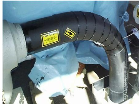
A flowline showing an M2 fitted to the inner bend radius
