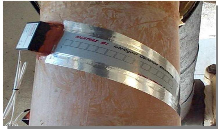
Hot Installation continuous @ 120 to 130 deg C prior to heat shield replacement
