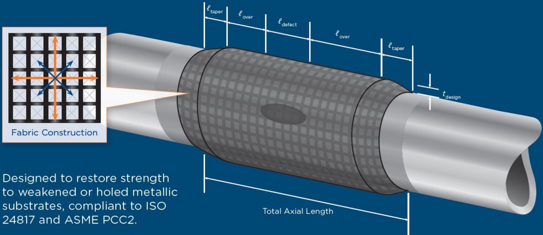
Designed to restore strength to weakened or holed metallic substrates, compliant to ISO 24817 and ASME PCC2.
