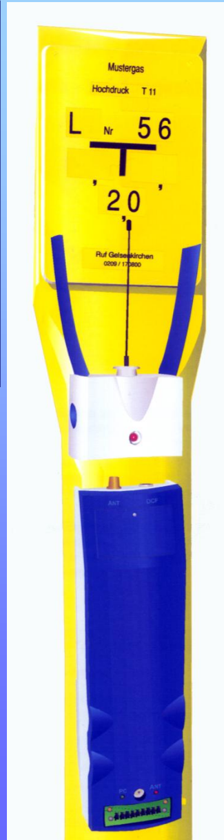
Complete system with sensor, radio antenna and extern charger
