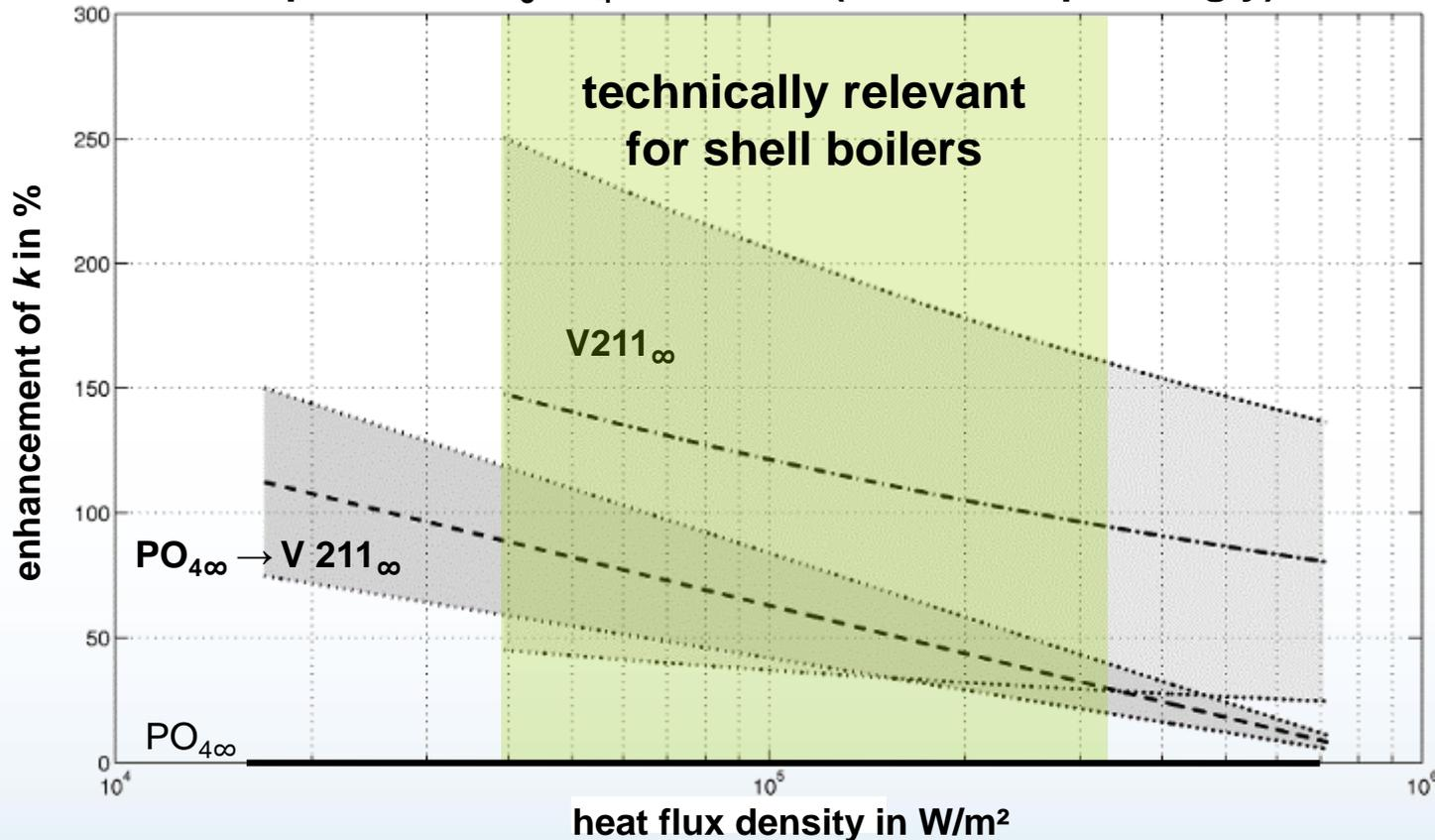
Shell boiler simulation at university of Rostock at „steady state“ conditions,  $p = 15$  bar
