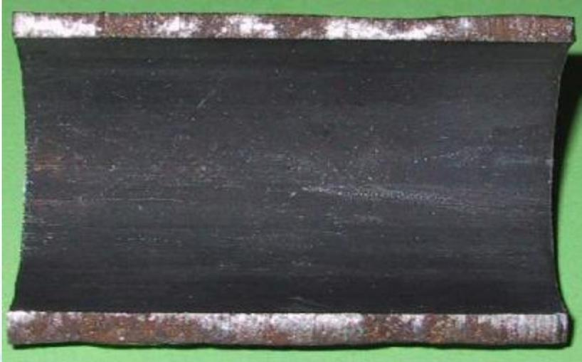
Magnetite Layer in Water-Tube Boiler
