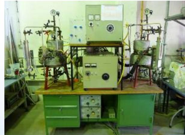
Shell boiler simulation at university of Rostock at „steady state“ conditions,  $p = 15 \text{ bar}$
