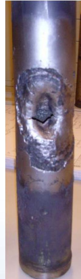
**Example of boiler tube failier**
