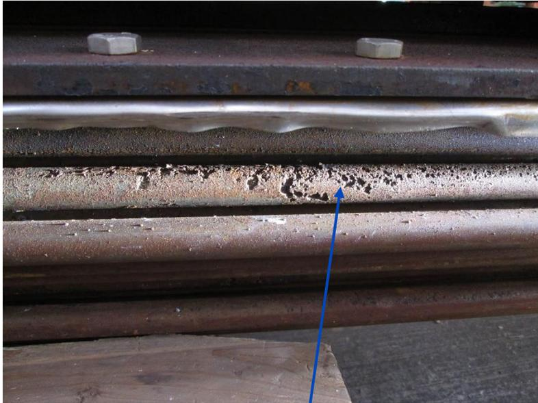
Slightly deep corrosion pits
