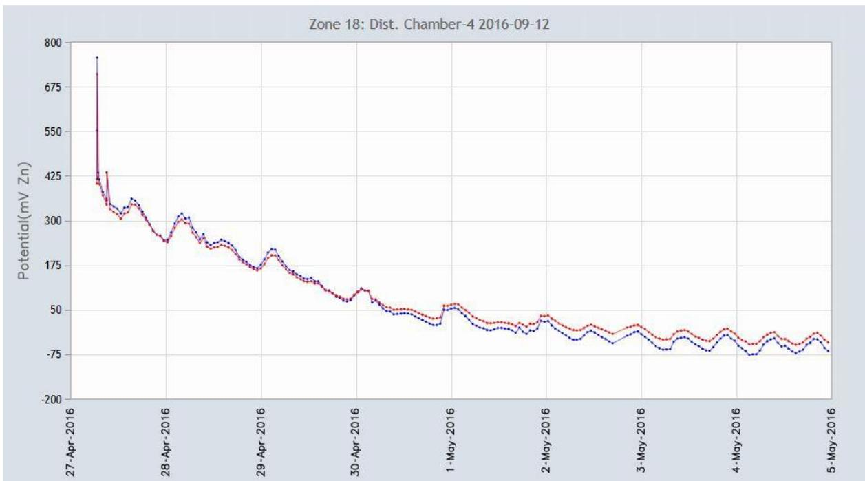
**Figure 14: Potential vs Time curve for Zone 18, Distribution Bay**
