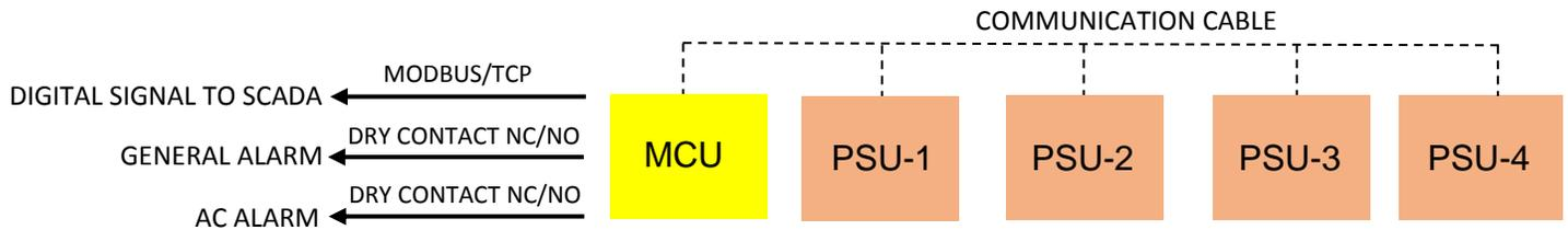
**Figure 11: Remote Monitoring and Control Architecture**
