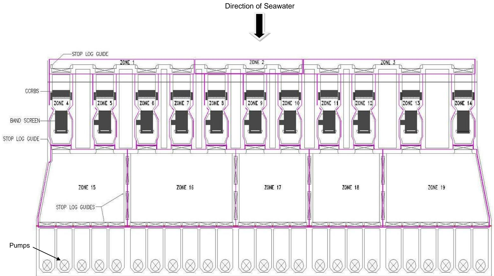
**Figure 1: Zoning arrangement of the CP system**
