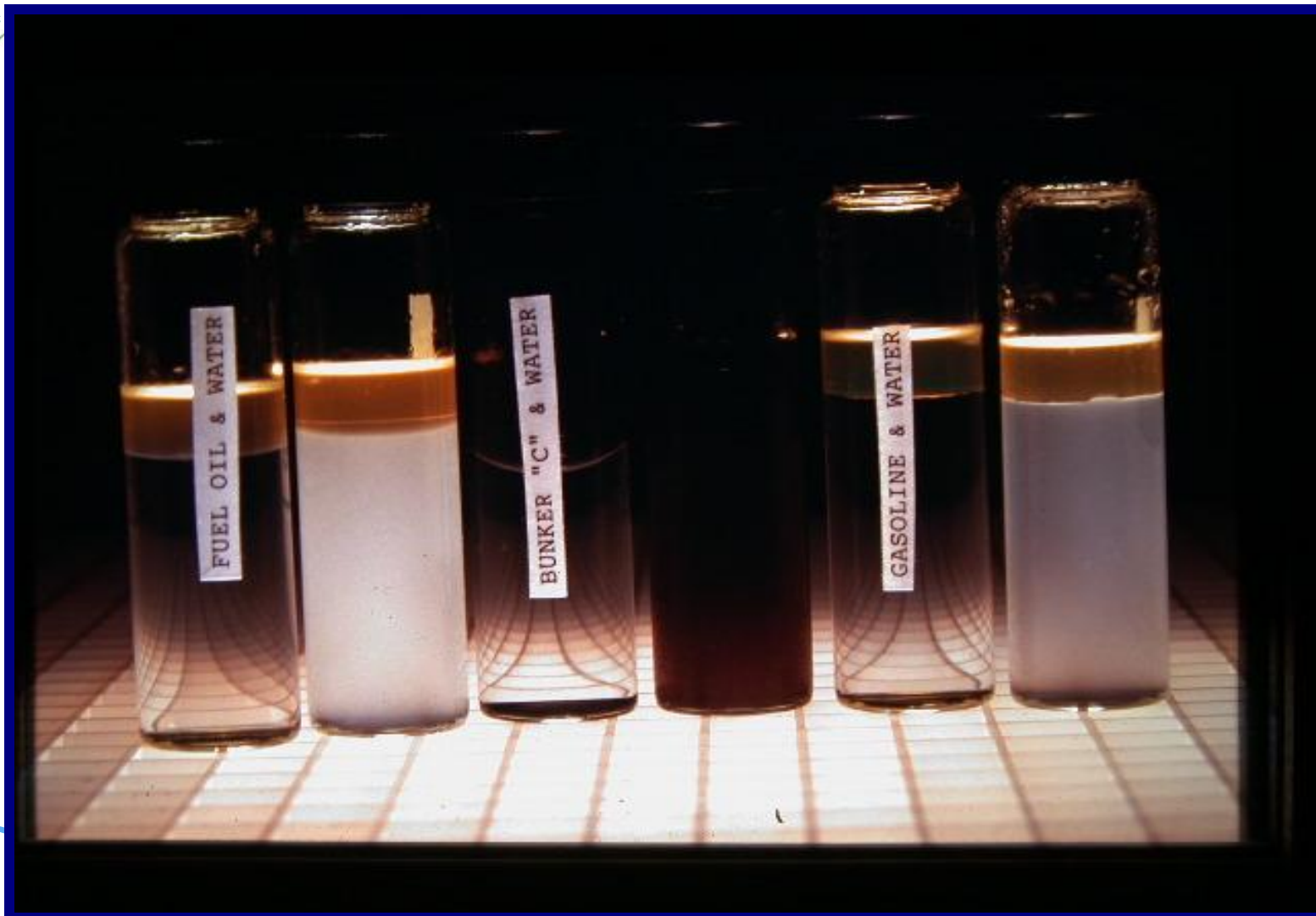
Fuel-oil – Bunker-C – Gasoline Dissolved In Water With Ivey-sol
