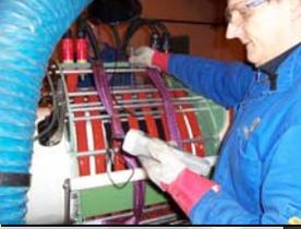
Force curing liquid epoxy with induction heat
