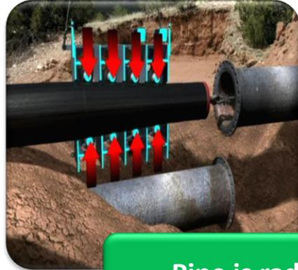
Pipe is radial compressed and installed in host pipe
