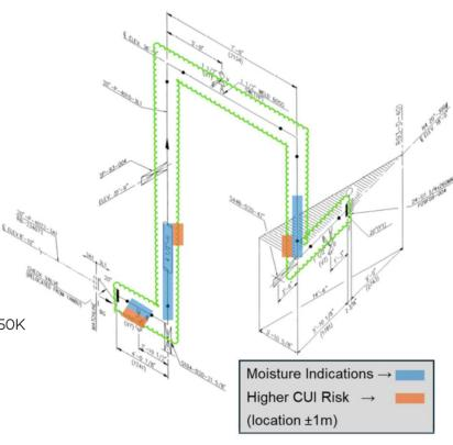
Example of the report generated from the CUI monitoring system showing marked-up isometric of an asset with moisture and CUI risk analysis
