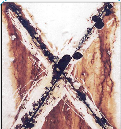
SC Epoxy - Two Coats (56% solids by volume)
