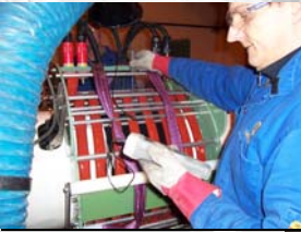
Force curing liquid epoxy with induction heat
