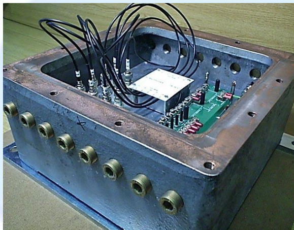
Or inside a cast iron flameproof enclosure (hazardous area use)
