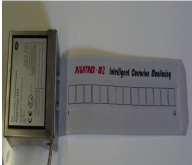
An M2 sensor fitted with armouring to the cable and a hazardous area gland
