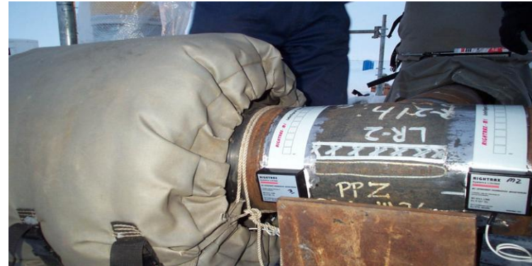
M2 sensors Fitted on Pipelines prior to insulation being reinstated
