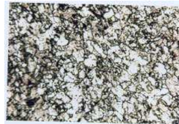
Fig 6 Microstructure of tube L at 100x magnification
